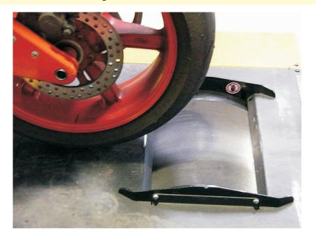
The heart of the system is the base dynamometer enclosure which holds the primary roll, front-wheel clamping assembly, and connections to the sensor box. The base dyno and all modules are suitable for pit installation.
